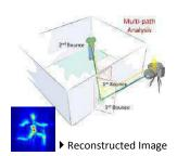
Using short laser pulses and a fast detector, the device can look around corners with no imaging device in the line of sight using scattered light and time resolved imaging.
