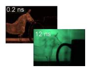
We repurpose a timeof-flight camera using coded illumination to recover time profiles of large-scale scenes to acquire multiple depths per pixel.
